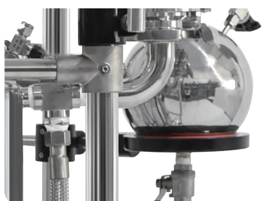
Collection flask: glass type or stainless steel type
